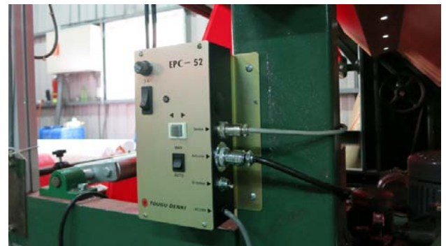
Controller Series 52 is installed on Hot Knife Slitting Machine by Wall-Mounted
